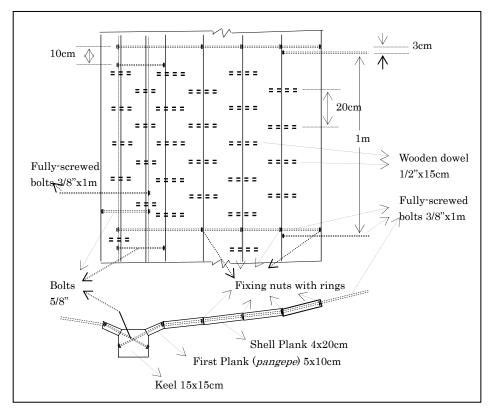
Fig. 5 The fishbone plank-fastening system
